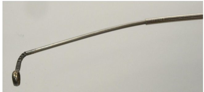
Fig. 1: Photograph of a wrist mounted to the tip of a concentric tube robot. The diameter of the wrist is 1.16 mm.
