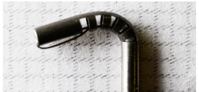
Fig. 8: The prototype was experimentally validated without the curette instrument (see Fig. 6) attached. The actuation tendon held open the last cutout of the wrist during the experimental trials, and the kinematics and statics models were calculated with n = 4 cutouts.
